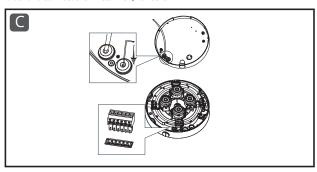
Position and screw each sensor at the desired angle. The sensors can be moved up, down, left, right, and rotated.
