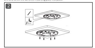
Pull each wire through the cable opening and connect. Then, install the camera onto the mounting plate. See optional procedures A and B to learn how to create a more secure attachment for these components and optional procedure C to learn how to install an alarm for the camera.
