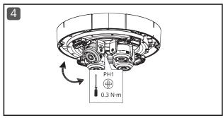
Install the camera's dome cover with the L-shaped Allen wrench provided. Remove the recyclable protective film and dispose of it.
